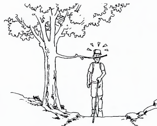
Figure 15-28. Objects that protrude into the pathway at a height greater than 685 mm (27 in) are difficult for pedestrians who use long white canes to detect.
